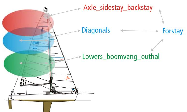
3) Tighten the lowers again with equal turns, looking up all the time too make sure the mast stays in column. Tighten so that they measure 20 on the LOOS B gauge. This will give pre-bend of 30cm
