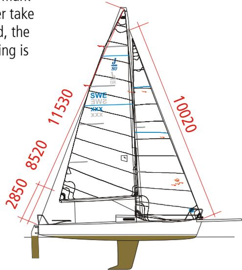
The Backstay is cut to 8520 and each leg shall measure 2850 mm.
